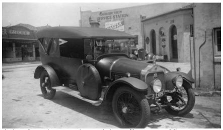
In 1908 Minerva adopted the Knight sleeve valve engine and prior to WW1 ran a wide range of sleeve valve engined cars ranging from 2.3 litres to 7.4 litres with the HH model. The silence of the motor added greatly to the car's reputation and it became the car of
